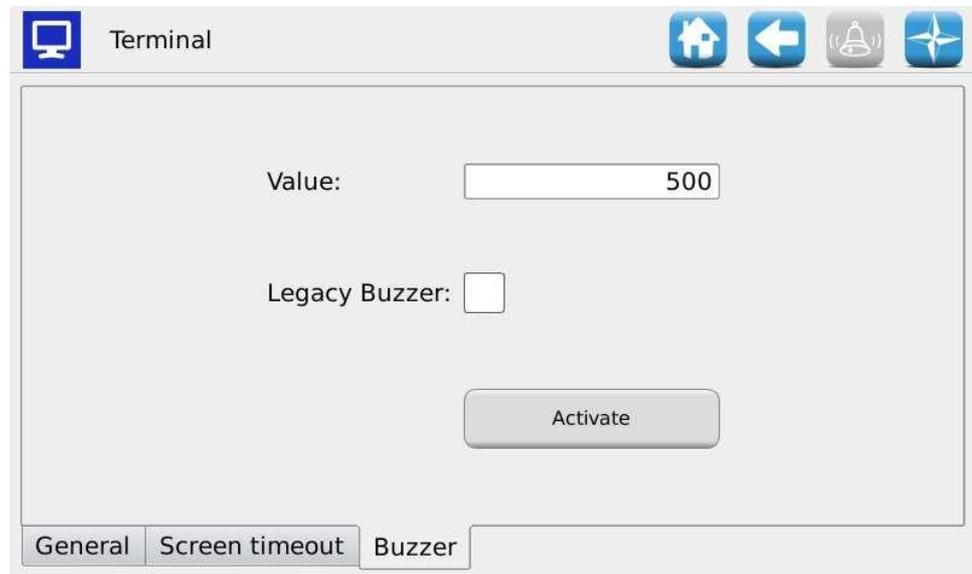
In this page it is possible to regulate the sound intensity of the console built-in buzzer. The values range from 50 to 1000.
