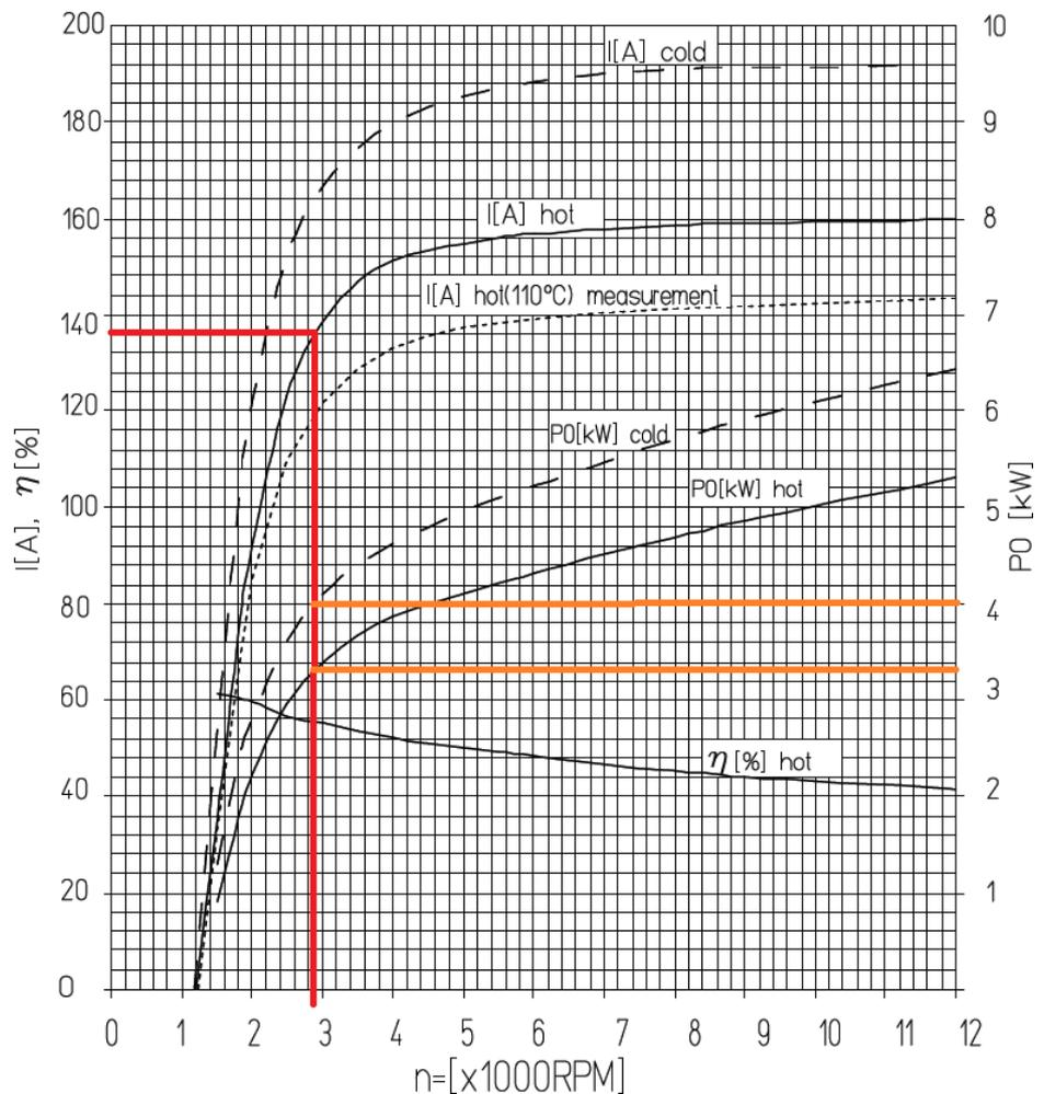
Figure 2-7 - Characteristic power curves for the alternator
