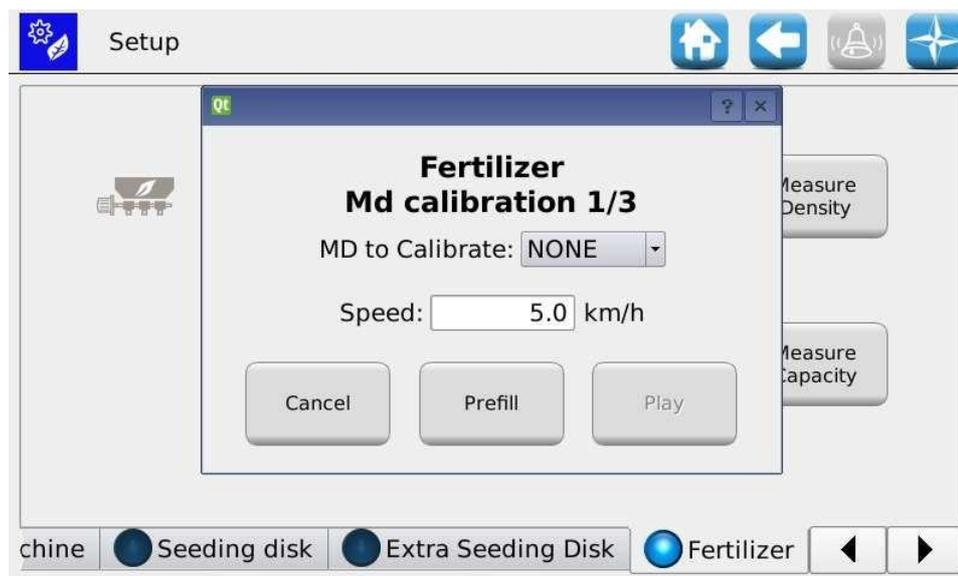
It is possible to select the motor to be calibrated as well as the prefill speed to be used.
