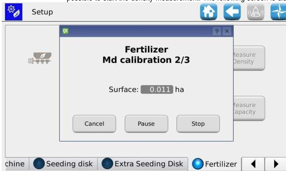
Let the motor run for at least 60 seconds (according to the machine settings) in order to get a good quantity of product in the bag (not less than 1/2 kg).
