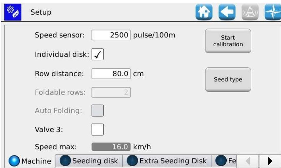
In the **Machine** Tab it is possible to activate the “Individual disk” function, which enables the “Extra Seeding Disk”. This tab allows to individually set the disk holes as well as the seeding distance for each row, by directly selecting the parameters of the row you want to modify.
