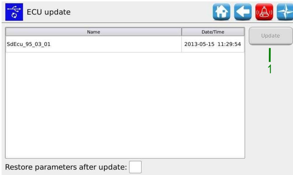
Selecting the desired software from the list and pressing the **1** button, it is possible to update the ECU software.
