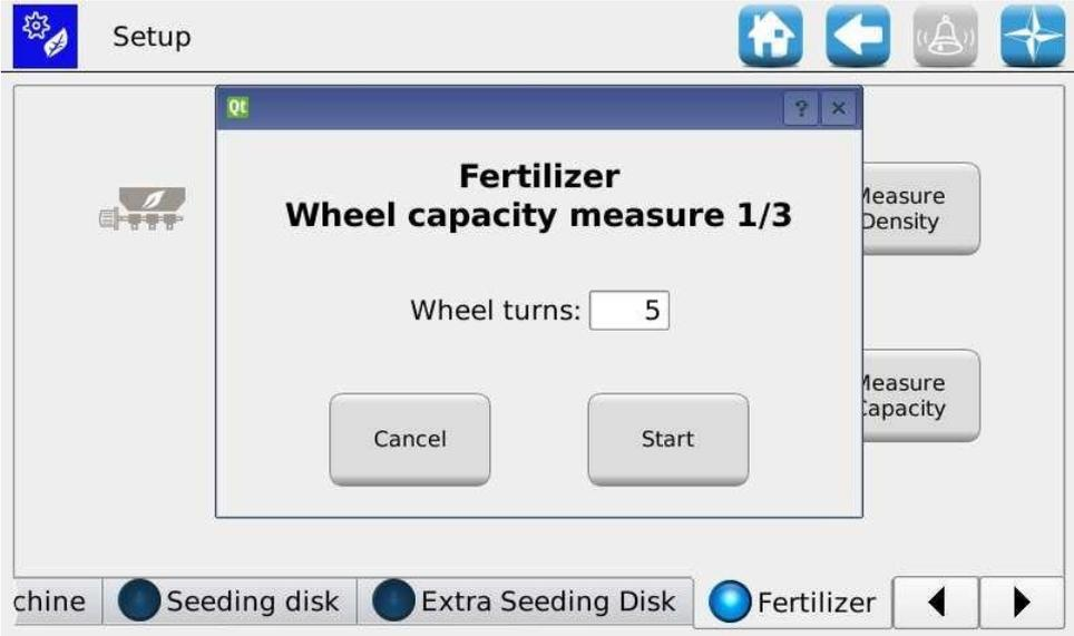
After setting a desired number of turns, the system will start up the motor related to the fertilizer 1 or the microgranulator 1. This operation can be done by measuring the spread quantity, dividing it by the number of turns and, if different from 1kg/dm<sup>3</sup>, even by the density, i.e:
