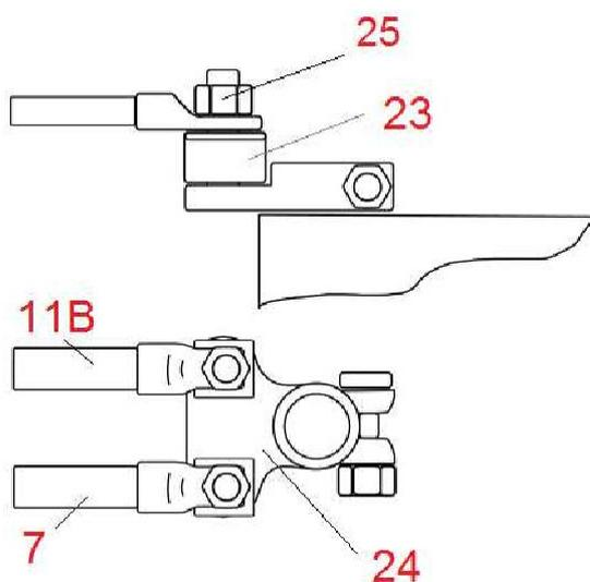
Figure 2-13 - Battery positive pole connection detail
