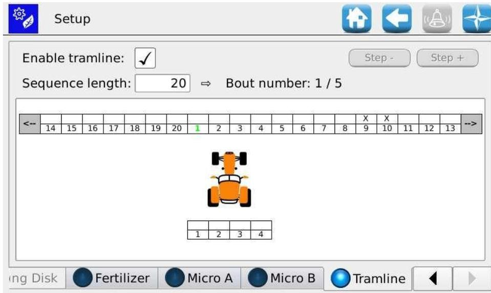
While analyzing the data, the system estimates that 5 steps will be necessary in order to complete the sequence. Thinking of the machine position on the field, we will see the machine “lifted” in transport position, with the left and right row markers “lifted”.
