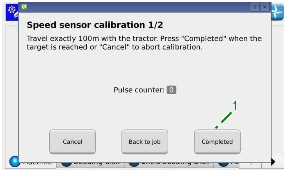
In order to calibrate the sensor, you need to trace a target line exactly 100m far from the actual tractor position, and to travel this 100m section at a moderate speed (5-9 km/h).
