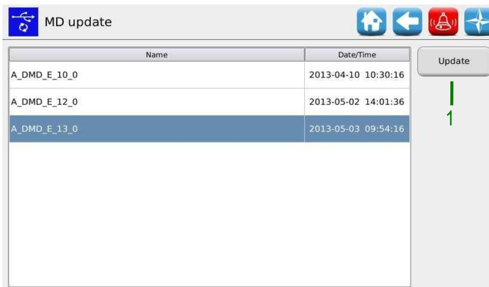
Selecting the desired software from the list, and pressing the **1** button, the following pop-up window is displayed where it is possible to choose the motor (and therefore the elements: seeding unit, fertilizers or micro-granulators) to be updated.
