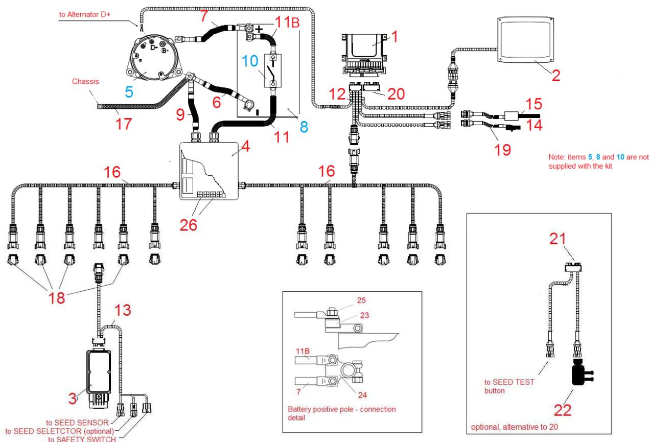
Figure 2-12 - Wiring diagram of the system with alternator
