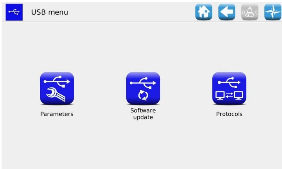
The accessible submenus on the operator's or OEM assistance level are “Software update” and “Protocol”.
