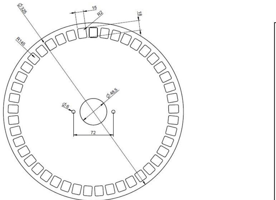
**Figure 2-9 - Example of cogwheel for speed sensor**
