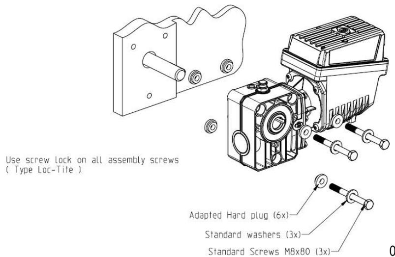
Figure 2-4 – Particulars for the geared motor fastening
