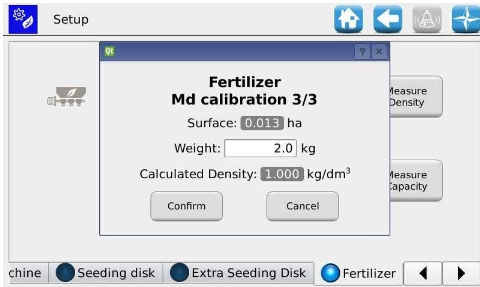
Input the weighted value and press Confirm. The value will be updated by the system in the Density field.
