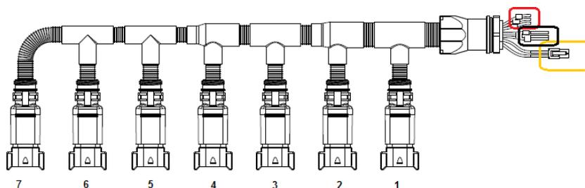
Figure 19 - 05R01373 cable – 7 outputs
