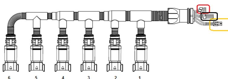
Figure 18 - 05R01372 cable – 6 outputs
