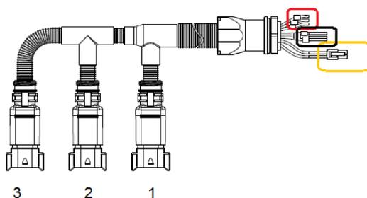
Figure 17 - 05R01404 cable – 3 outputs
